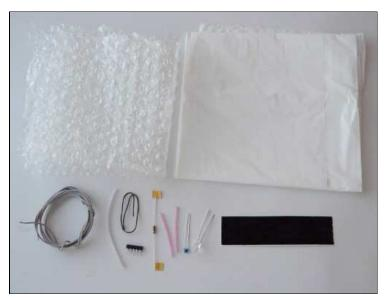
The basic "glowing ghost kit" contains the basic parts to build the ghost. The included white LED produces a very bright white light. In addition to this kit we need the atmega8 microcontroller and some batteries or a little DC power supply, 4.5V to 5.5V (Ericsson mobile phone chargers provide 5V DC).
