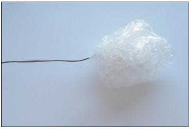
We wrap a very bright white LED in bubble padding foil. This foil will diffuse the light. Using transparent adhesive tape the bubble foil is wrapped up and forms a little ball. A litte bit smaller than a tennis ball. This little ball is the head of the ghost.
