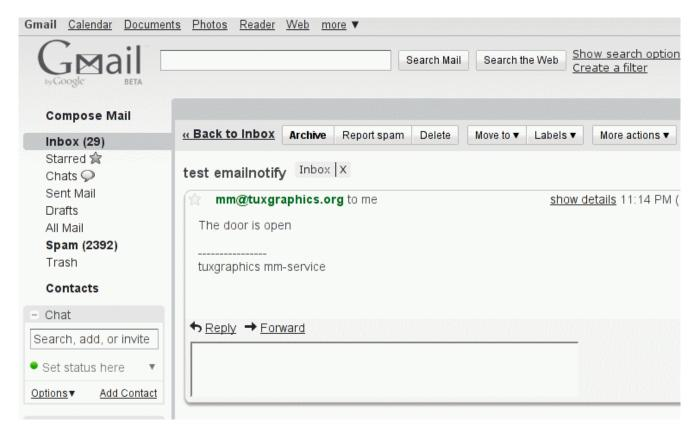
test\_emailnotify.c has also a timer to prevent flooding with mail. A second mail is sent no earlier than 3 minutes after the frist mail. The ethernet board runs in addition a web server so you can remotely monitor statistics and stop email notifications:
